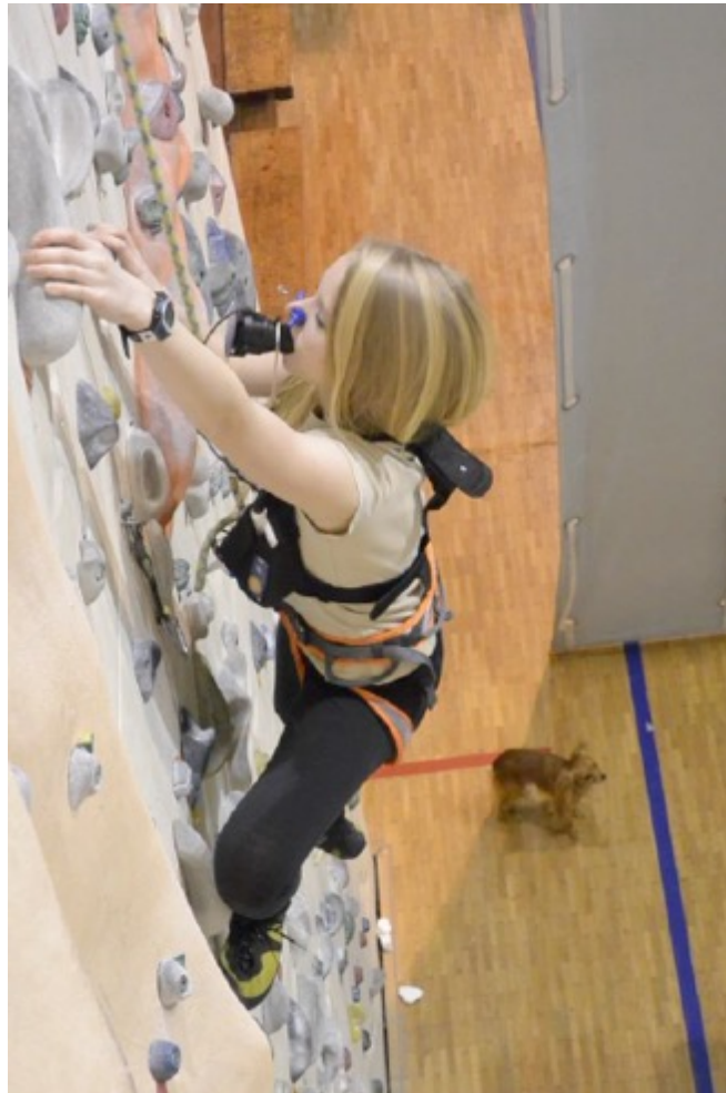
Figure 1. Energy expenditure measurement in climbing using a portable gas analyzer (Metamax3B, Cortex, Germany) (Panackova et al., 2014).
